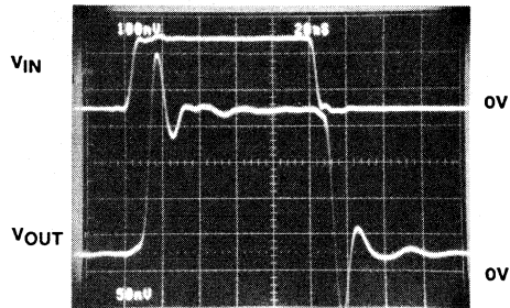
SMALL SIGNAL RESPONSE Vertical Scale (Volts: 100mV/Div.) Horizontal Scale (Time: 50ns/Div.)
